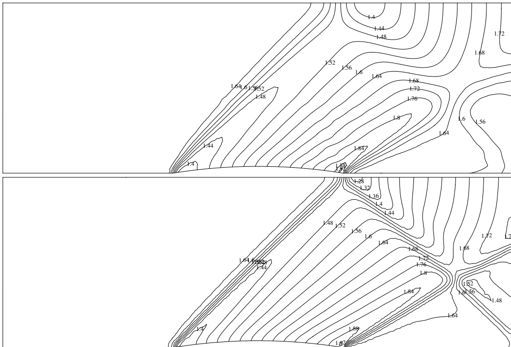
Fig. 13. Channel with a bump, supersonic flow case. Mach number isolines. First-order scheme (top) and the scheme with linear reconstruction (bottom). Vertex-based reconstruction was applied in the density and in the momentum equation, and the cell based reconstruction was used in the energy equation.
